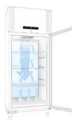
cabinet. When combined with the Gram BioLine air distribution system, it also ensures even better temperature stability inside the cabinet.
