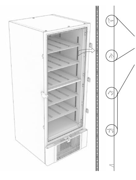
**I-16\*:** Mount the shelf support clips to the wall rails, using the numbering on the wall rails to determine the right shelf height. Finally placing the shelf on the supports on the support clips.
