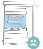
Conventional refrigerator with evaporator in the storage space, evaporating refrigerant lowers temperature by absorbing heat and transferring it outside the cabinet.
