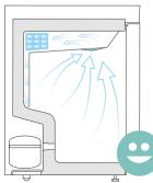
BioCompact 210 Refrigerator with a finned tube evaporator enables forced air distribution inside the storage chamber. Thereby evenly distributing cold air throughout, enhancing temperature stability and uniformity.
