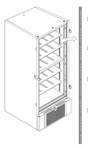
I-16\*: Mount the shelf support clips to the wall rails, using the numbering on the wall rails to determine the right shelf height. Finally placing the shelf on the supports. Please note that the pronounced lip on the shelf must face outwards, as shown in the illustration.
