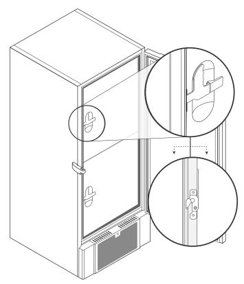
I-18\*: The inner doors are locked when the door lever clicks in place and sits flush up against the inner door.
