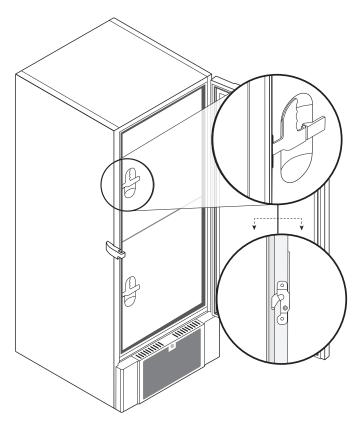
**I-18\*:** The inner doors are locked when the door lever clicks in place and sits flush up against the inner door.
