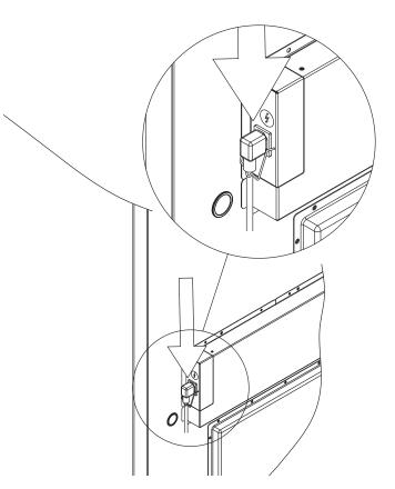
The appliance must be connected to the external power supply using a suitable device which mechanically prevents the plug and socket from being separated unintentionally.
