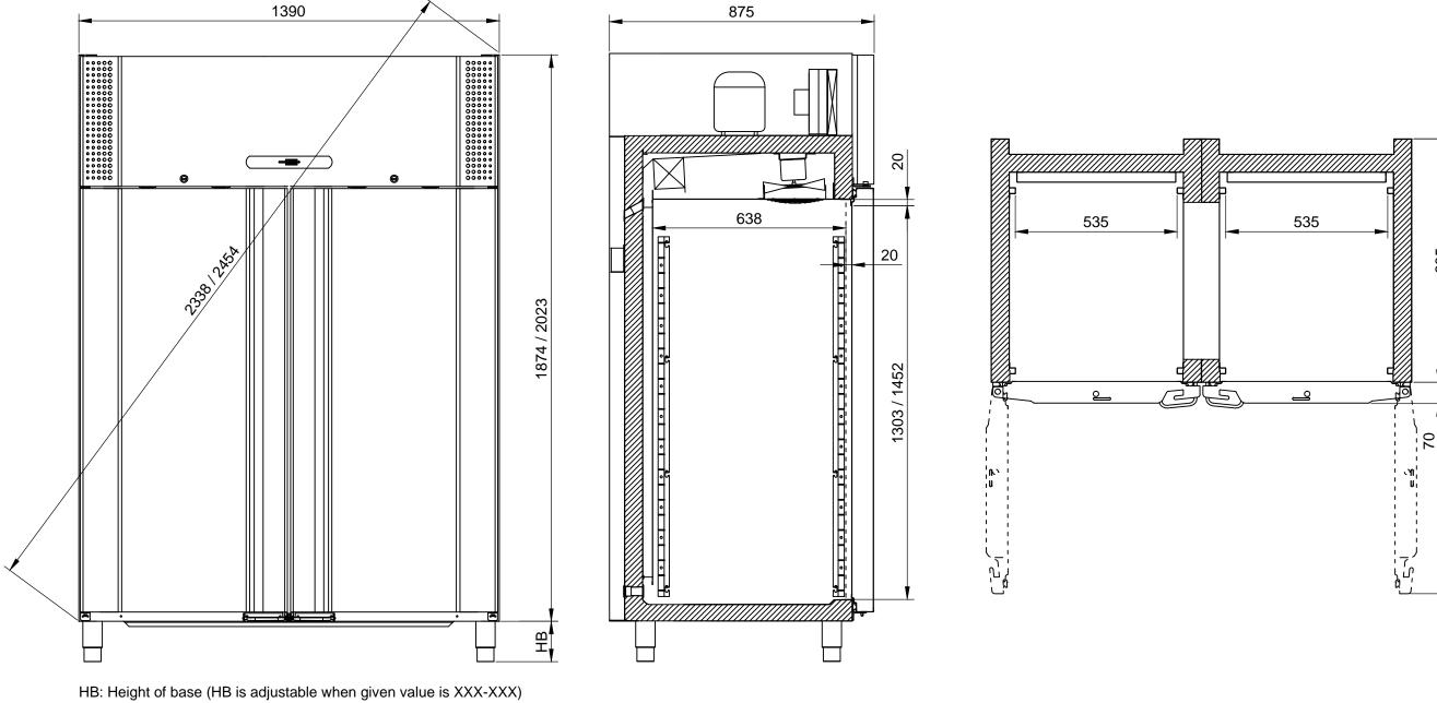
Note: 20 mm air passage is 25 mm when cabinet is equipped with draught shield (option 70)
