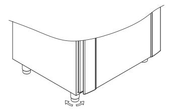
**I-10\*:** For cabinets equipped with castors, the floor must be level to ensure stable positioning and safe use. When the cabinet is positioned, the 2 front castors should be locked.
