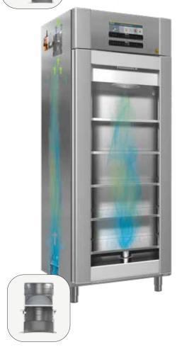
Ambient air is drawn into the cabinet interior through a check valve when the damper opens, equalising the pressure in the interior thereby flushing out potentially contaminated air.
