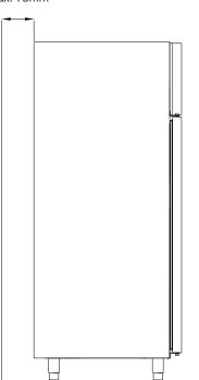
Do not cover the upper part of the cabinet if it has a top mounted compressor (applies to BioBlood 500, 600/660 and 1270/1400).
