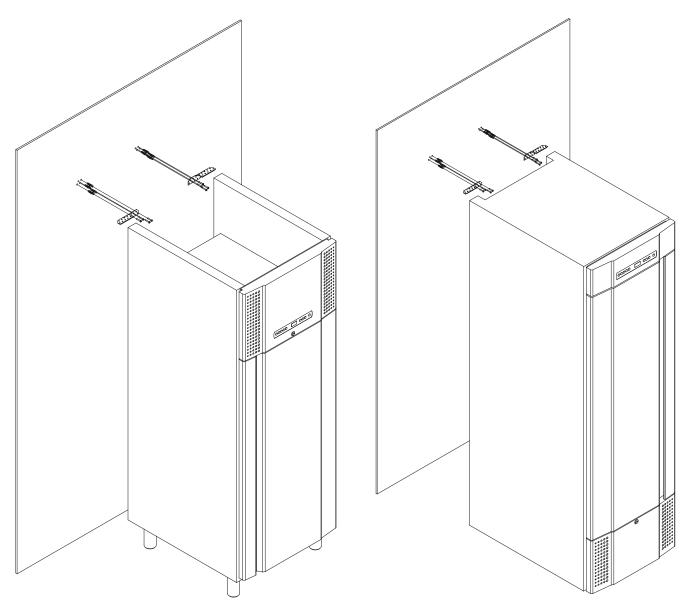
The anti-tilt brackets must be fitted when installing the cabinet, ensuring that the users, surroundings and stored items are not damaged by a tilting cabinet.
