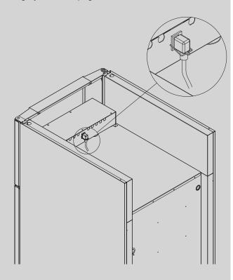
The appliance must be connected to the external power supply using a suitable device which mechanically prevents the plug and socket from being separated unintentionally. The connection must be labelled:
