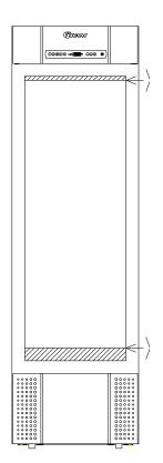
Items placed on the bottom of the cabinet will cause the air circulation to be impeded, which reduces the cabinets performance.
