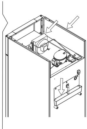
It is recommended that the re-evaporation tray is checked regularly for foreign objects and cleaned accordingly.
