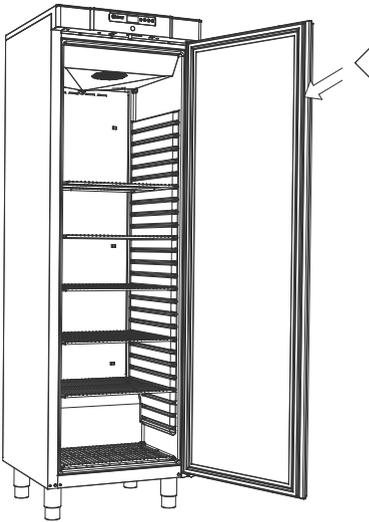
The door gasket should be cleaned regularly with a mild soap solution.
