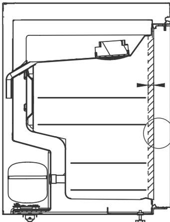
There must be a 20 mm gap between the inner part of the door and the stored items, to enable airflow at the front of the cabinet.
